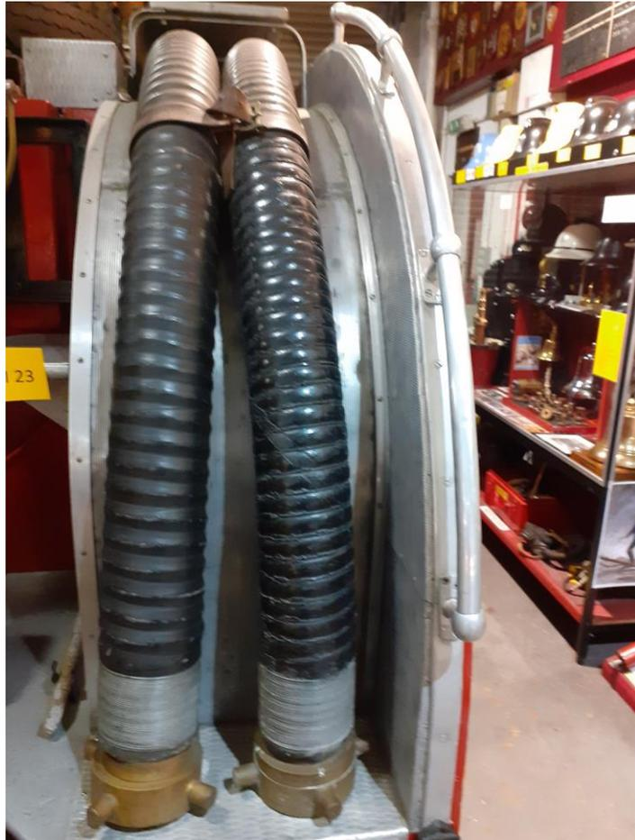
Suction hose, carried on a fire appliance from the 1950s. Modern suction hose differs only slightly from this type of hose.
