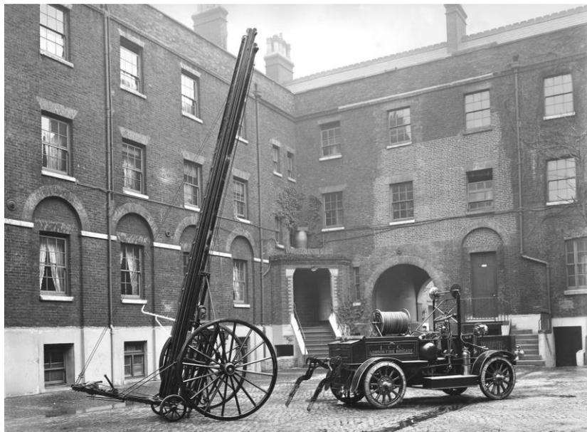
An early Merryweather Motor Escape Van, showing the 'First Aid' hose reel. The water tank is under the driver's seat. (Photo courtesy of the London Fire Brigade).
