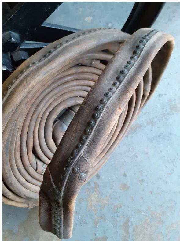
Leather fire hose, dating from the 1890s, showing its construction.
