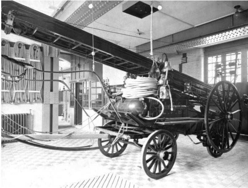
A Horsed Escape Van of the London Fire Brigade from around 1910, showing the 'First Aid Hose' coiled up next to the Coachman's seat. The water was supplied from the large pressurised copper water tank on the foot-board. (Photo courtesy of the London Fire Brigade).
