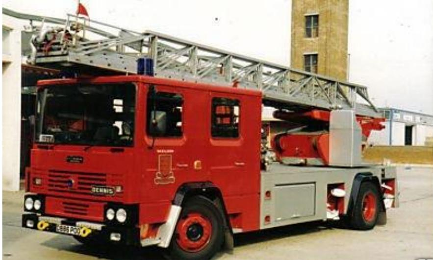
The ladder set from the Clacton AEC Mercury/Merryweather on its new Dennis DFD 133 chassis in 1986. (EFM Collection)
