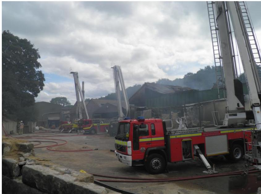
Three Hydraulic Platforms following fire-fighting operations at a major fire. The folding booms are clearly shown. Note the span of the outrigger jacks. (Derbyshire Fire and Rescue Service)
