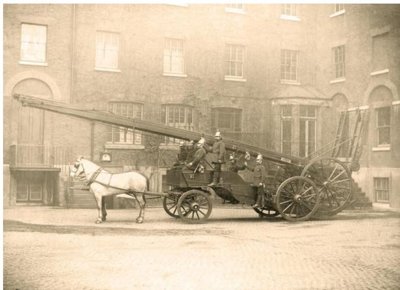
A London Fire Brigade 'Long Ladder'. These ladders could reach 70ft (21m) high but weighed in at 2 tons and required a crew of five or six firemen to operate. Notice the heavy construction of the 'chariot style' carrying vehicle. (Photo courtesy of the London Fire Brigade [LFB] Museum)
