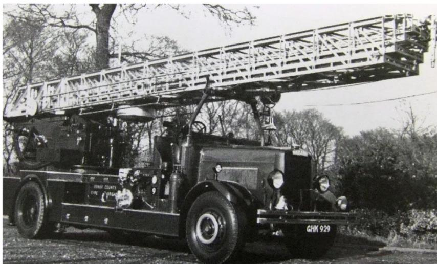
Clacton Fire Brigade's 1938 Leyland Metz 100ft (30m) T.L. Note the extremely long overhang of the ladder at the front of the vehicle and the large quadrants at the rear of the ladder. Seen in post 1948 ECFB livery. (EFM Collection)
