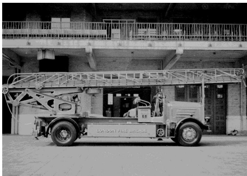
A London Fire brigade Dennis/J. Morris/ Magirus 105ft (32m) T.L. of 1937. The hydraulic elevating ram can be seen below the rear fulcrum frame under the rear of the ladder. The small wheel by the front wheel-arch controls a ground jack. (Photo courtesy of the LFB Museum.)
