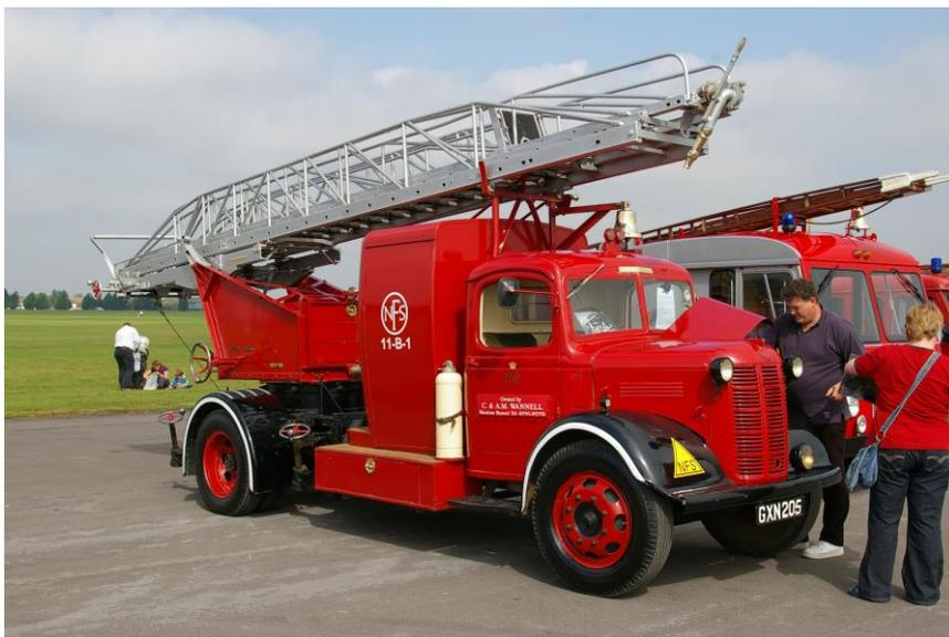
Austin K4/ Merryweather 60ft(18m) hand operated turntable ladder. Shown in its 1947 post WW2 NFS red colour scheme, this vehicle served at NFS Station 11.B.2 Brentwood. Note the large 'pull down' elevating lever at the rear of the ladder. (M Beale Collection.)
