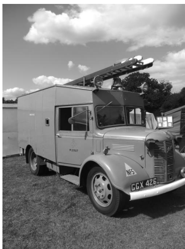
An Austin K3 ATV as used by Chelmsford's NFS to tow trailer pumps post 1941 (Author's Collection)
