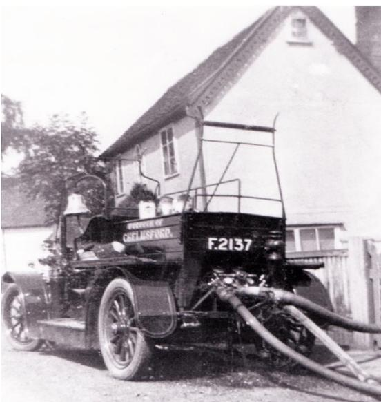
Rear view of Chelmsford's Panhard motor fire engine fitted with a Dennis pump and ladders. c1920 (EFM archive)
